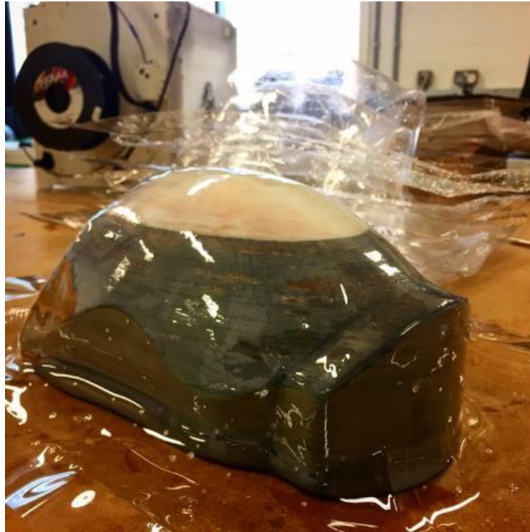
Figure 6 - Vacuum Formed Visor
