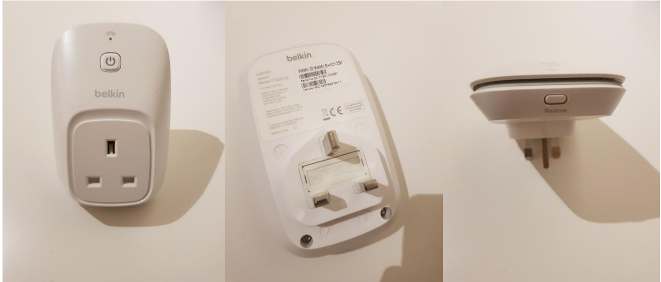
Figure 5: Front, Back and Restore Button of Belkin WeMo Smart Plug
