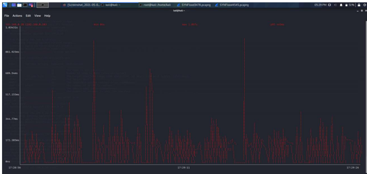
Figure 30: Graphical Representation of Ping During SYN Flood Attack on Port 4545
