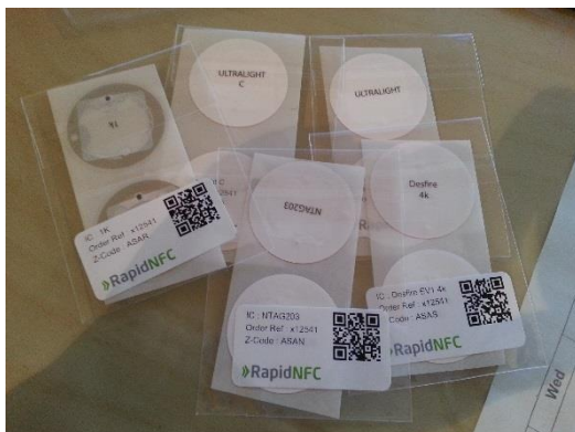
Fig [3] - This Image shows several different types of NFC tag as I plan to test to see which type will be most efficient for my application. Each chip can store various amounts of data and has different scan strengths which mean they can be scanned from a limited distance- this could prove useful in the gym environment.
