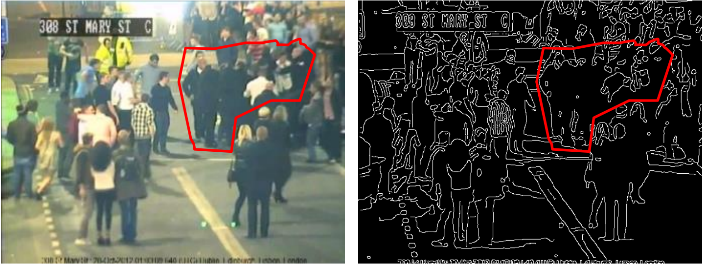
FIGURE 16: HIGHLIGHTED AREA OF VIOLENCE SHOWS A LOW NUMBER OF DETECTABLE EDGES
