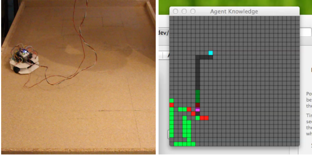
Figure 28: An example of results produced by the robot as it maps out an empty environment. These results demonstrate how the movement functions of robot are imprecise and inconsistent.
