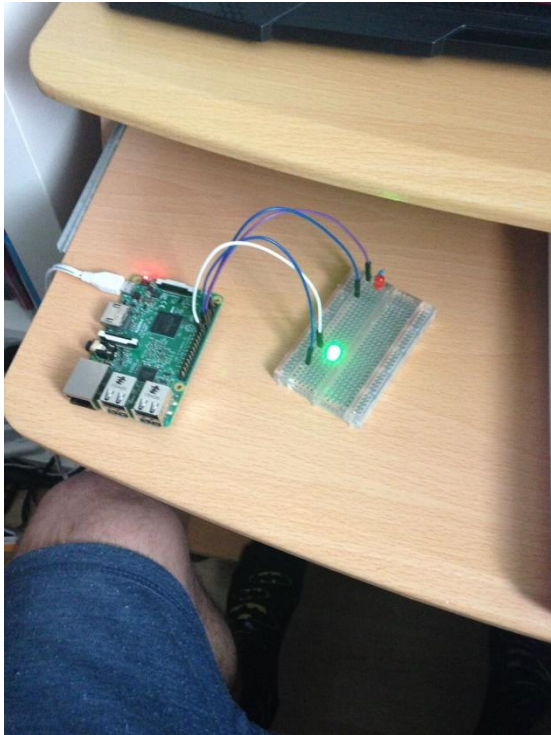
FIGURE 4.13 – GREEN LED TURNING ON WHEN POLICY IS ACCEPTED
