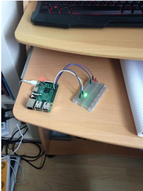
FIGURE 5.7 – RASPBERRY PI LIGHTING UP THE GREEN LED AFTER SUCCESSFUL POLICY
