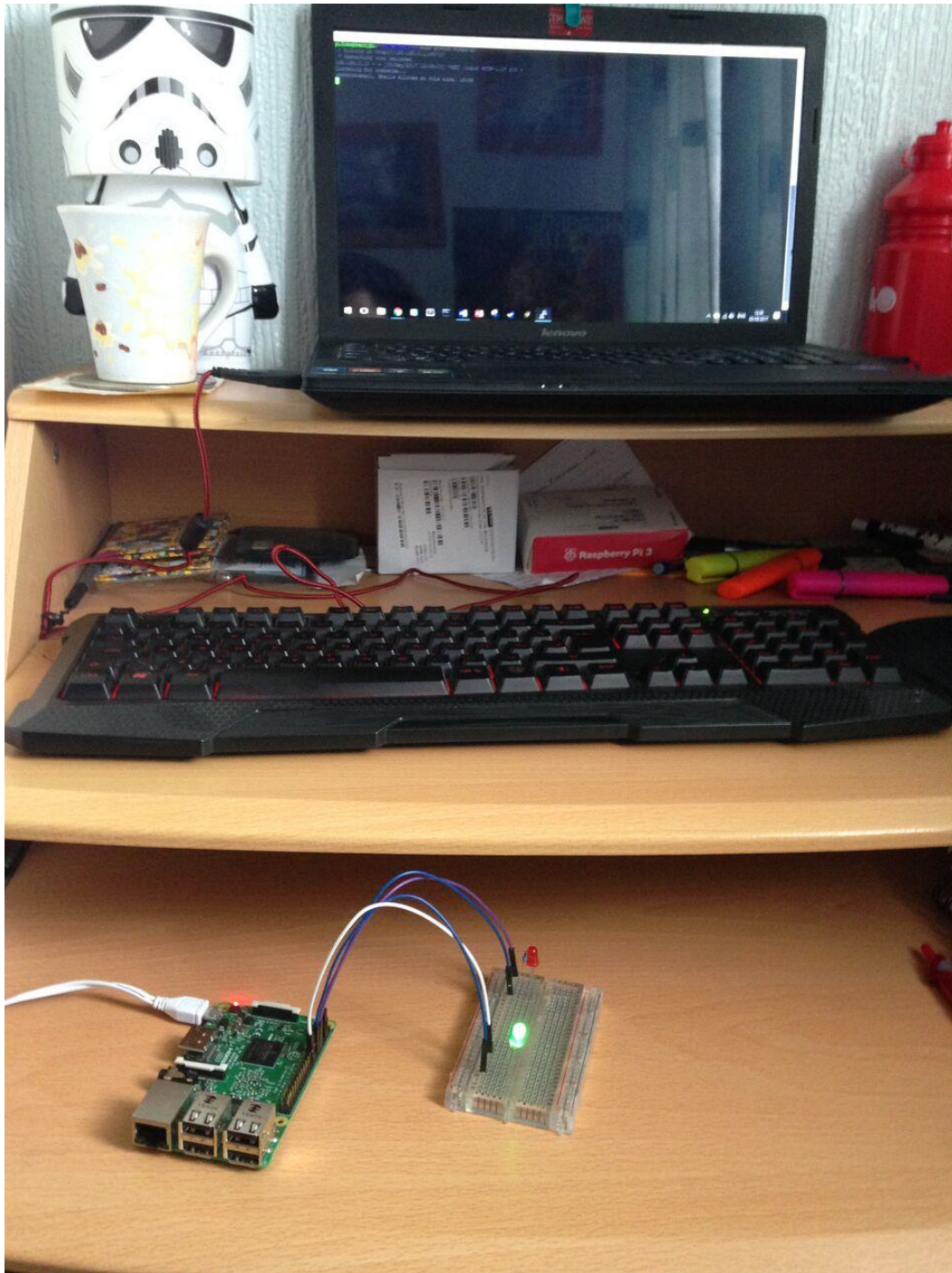
Setup of the solution, laptop running putty to control the Raspberry Pi, the Raspberry Pi connected and running. The Pi LED is green due to a successful criteria being met for the policy.
