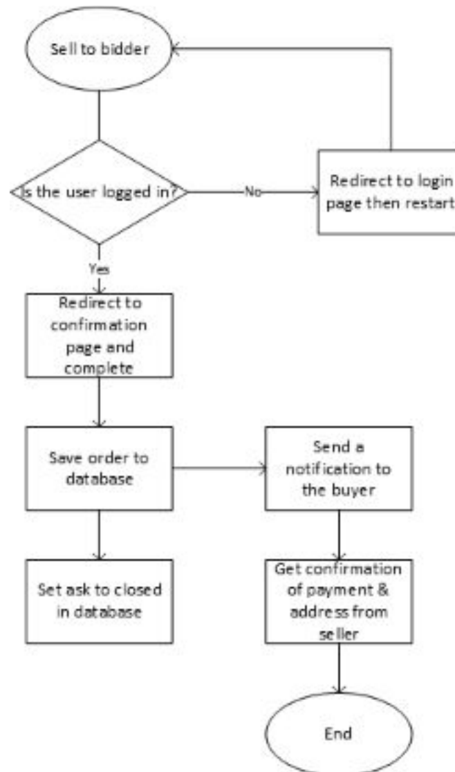
Figure 3.3: Flowchart for selling a product to another user for the user's previously placed bid.
